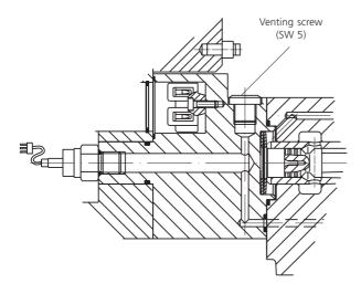
With pressure command set and lowered supply pressure, carefully open the venting screw by turning it **approxima-tely one turn**. The entrapped air should escape now together with hydraulic fluid. Wait until no more air bubbles can be seen in the oil. Then close the venting screw and torque it to **10 Nm**.
