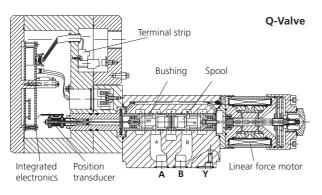
drive is a permanent magnet linear force motor which actively strokes the spool from its spring centred position in both directions. The closed loop spool position electronics and pulse width modulated (PWM) drive electronics are integrated into the valve. This permits control of the valve directly from, for example, a machine control without the use of additional interface electronics.
